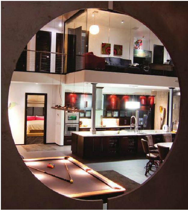
Glass walls above baffle noise when the lower level is used for entertaining.
